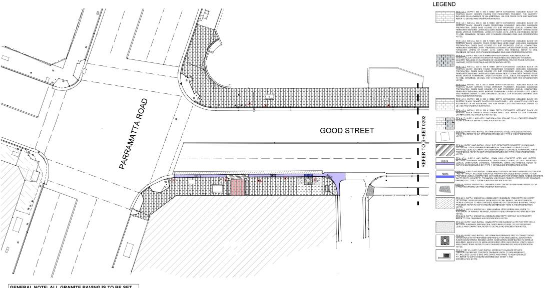
GENERAL NOTE: ALL GRANITE PAVING IS TO BE SET OUT FROM SET OUT PLAN, DETAILS AND SPECIFICATION NOTES. DO NOT SET OUT FROM GENERAL HATCH
