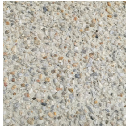
EXPOSED AGGREGATE CONCRETE PAVING Throughout proposed works
