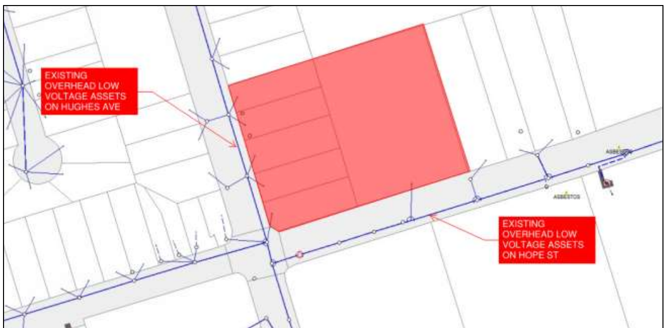
Figure 5 – LV infrastructure in the vicinity of the Site (source: Endeavour Energy)
