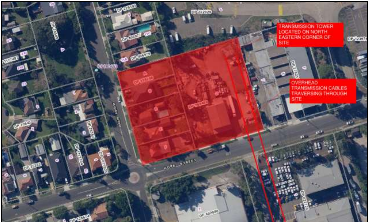
Figure 6 – HV Transmission in the Site (source: Six Maps)
