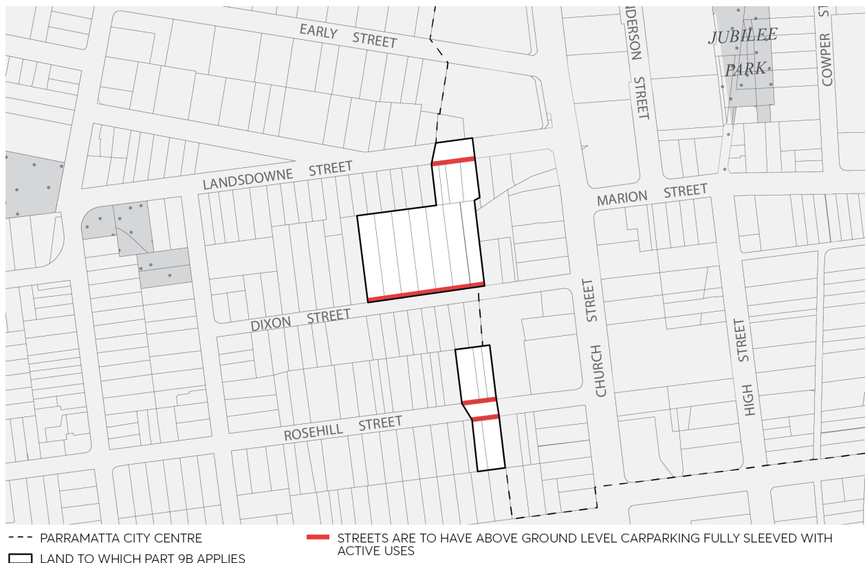
Figure 9B.4.3 – Above Ground Carparking Frontage Treatments
