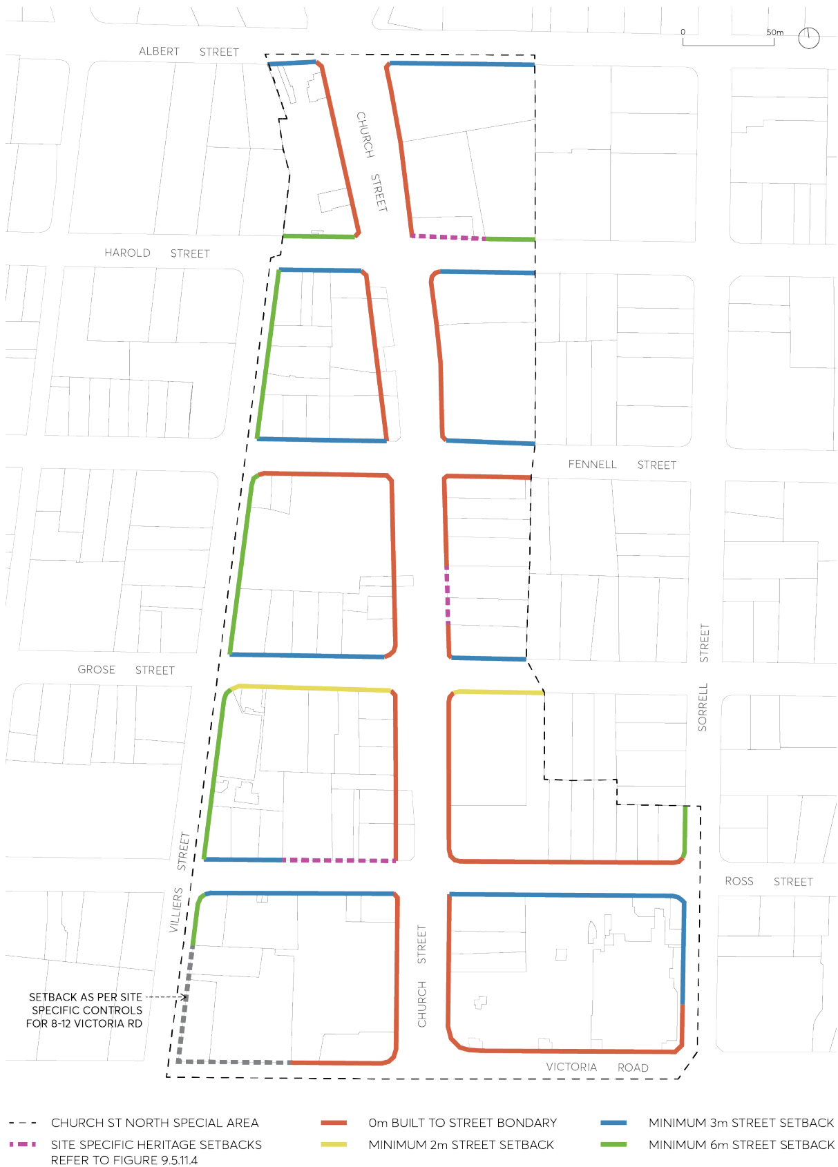
Figure 9.5.11.3 – Church Street North Special Area Building Setbacks
