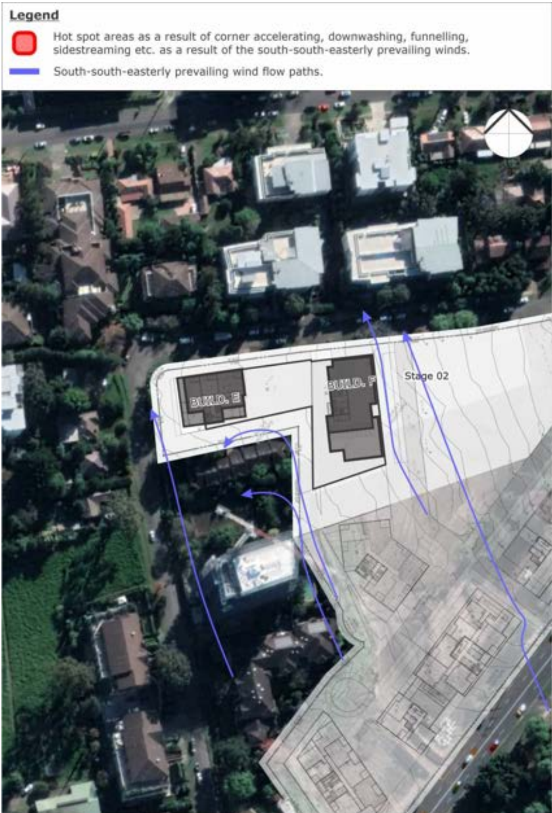
Figure 10: South-South-Easterly Wind Flow Hotspots Future Built Form in Stage 02 - Ground Level Plan
