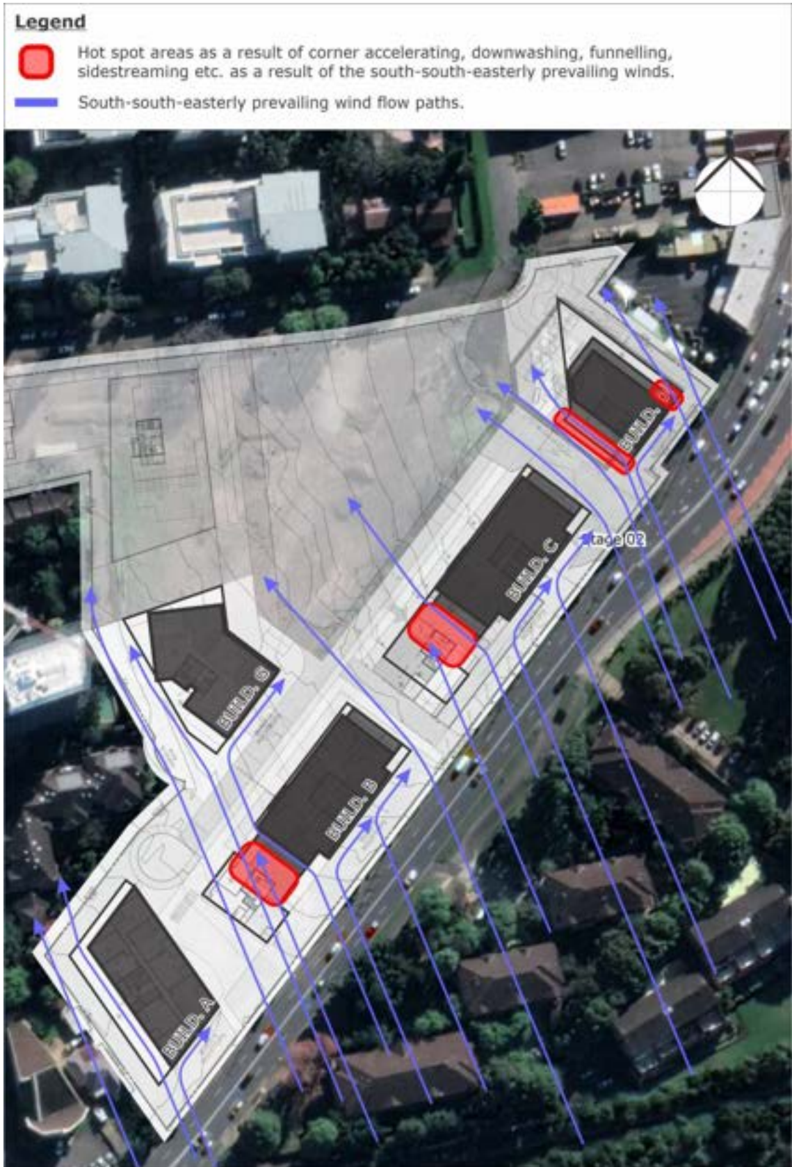
Figure 9: South-South-Easterly Wind Flow Hotspots Future Built Form in Stage 01 - Podium Level Plan
