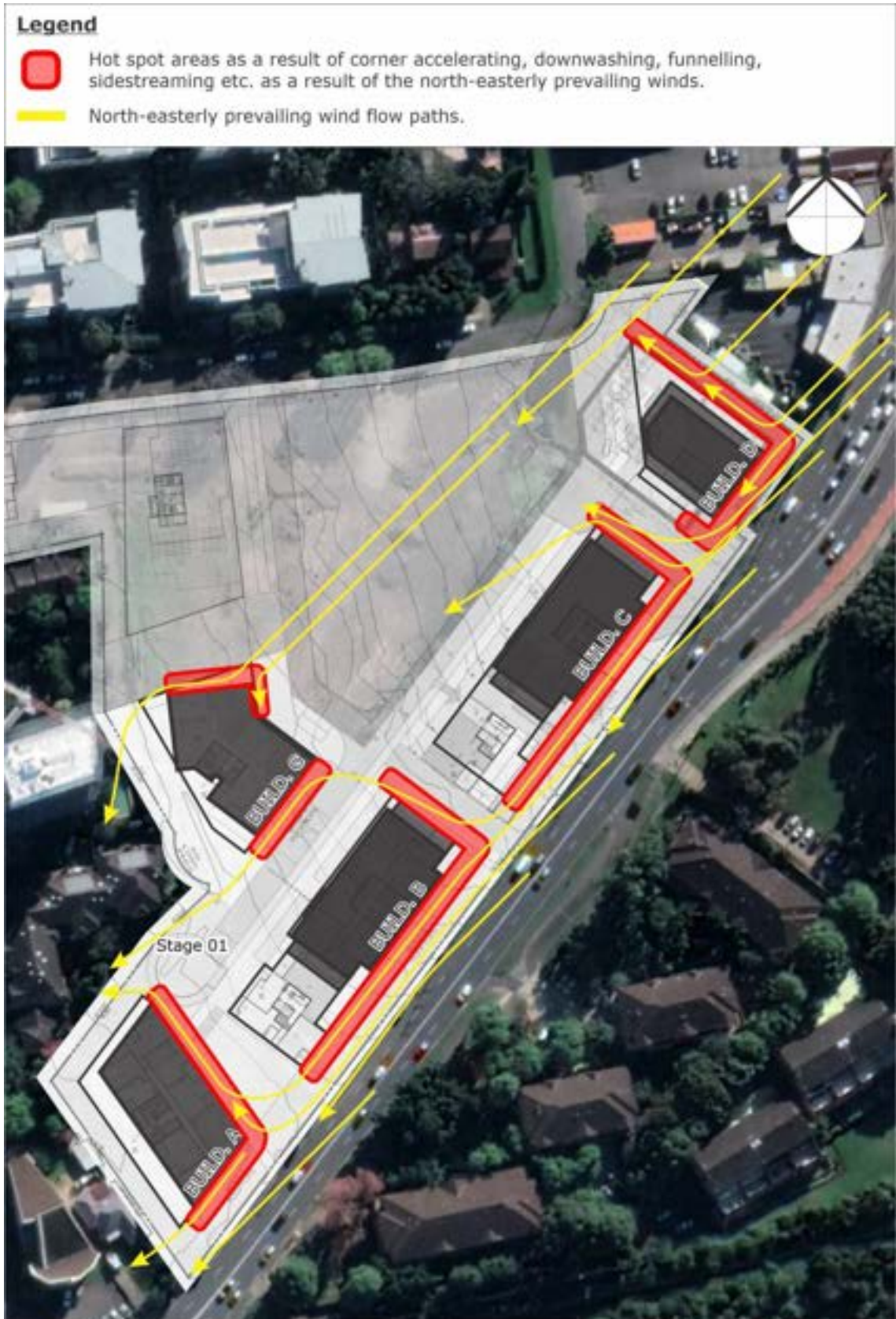
Figure 4: North-Easterly Wind Flow Hotspots Future Built Form in Stage 01 - Ground Level Plan
