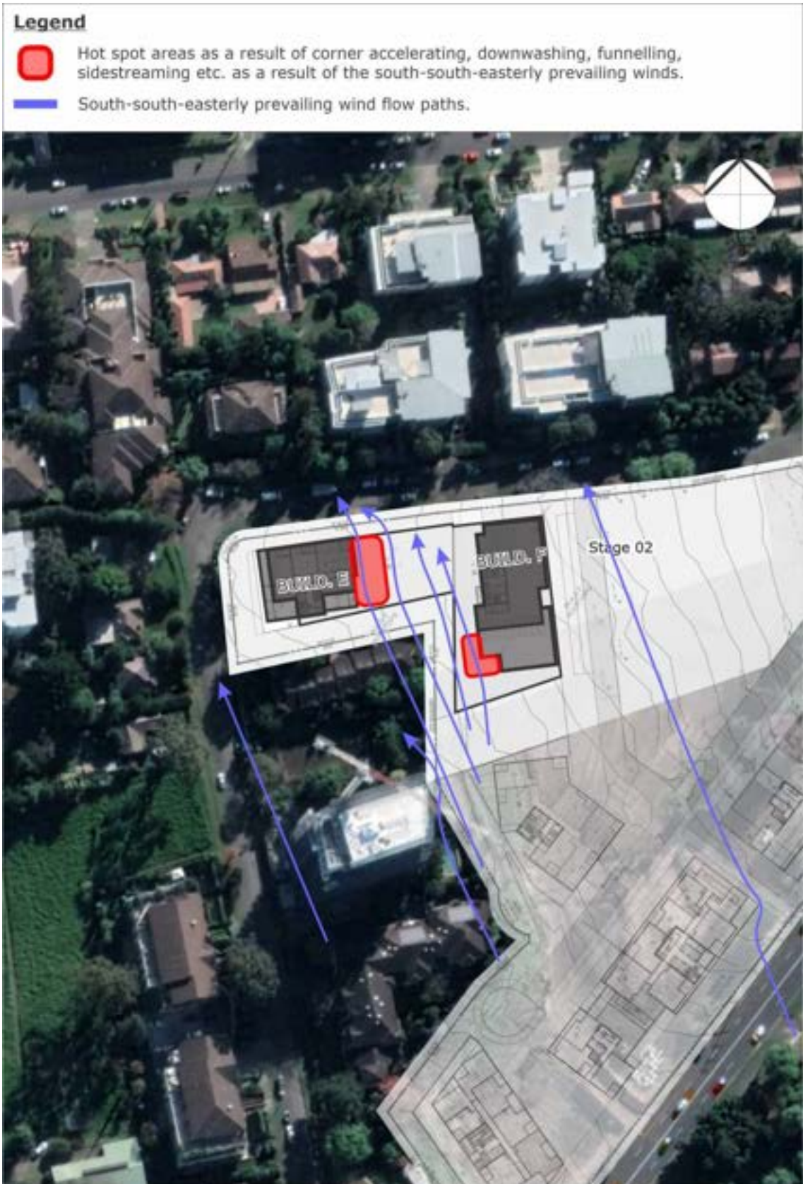
Figure 11: South-South-Easterly Wind Flow Hotspots Future Built Form in Stage 02 - Podium Level Plan
