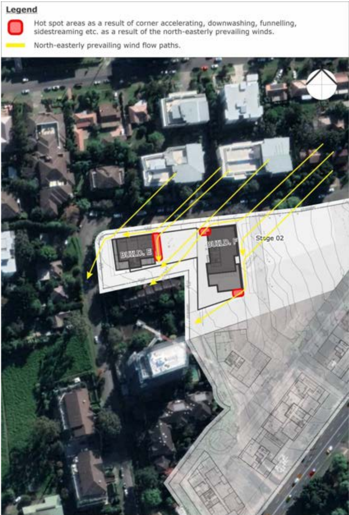
Figure 7: North-Easterly Wind Flow Hotspots Future Built Form in Stage 02 - Podium Level Plan
