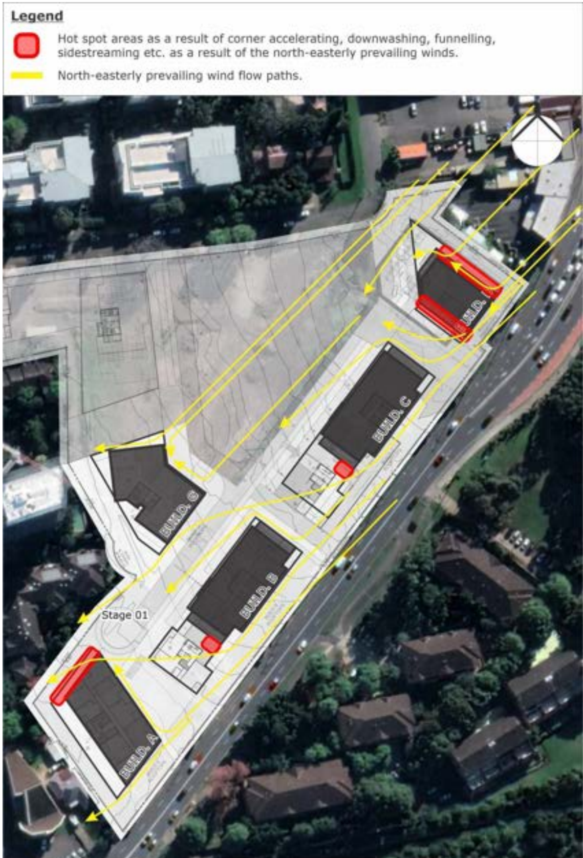
Figure 5: North-Easterly Wind Flow Hotspots Future Built Form in Stage 01 - Podium Level Plan
