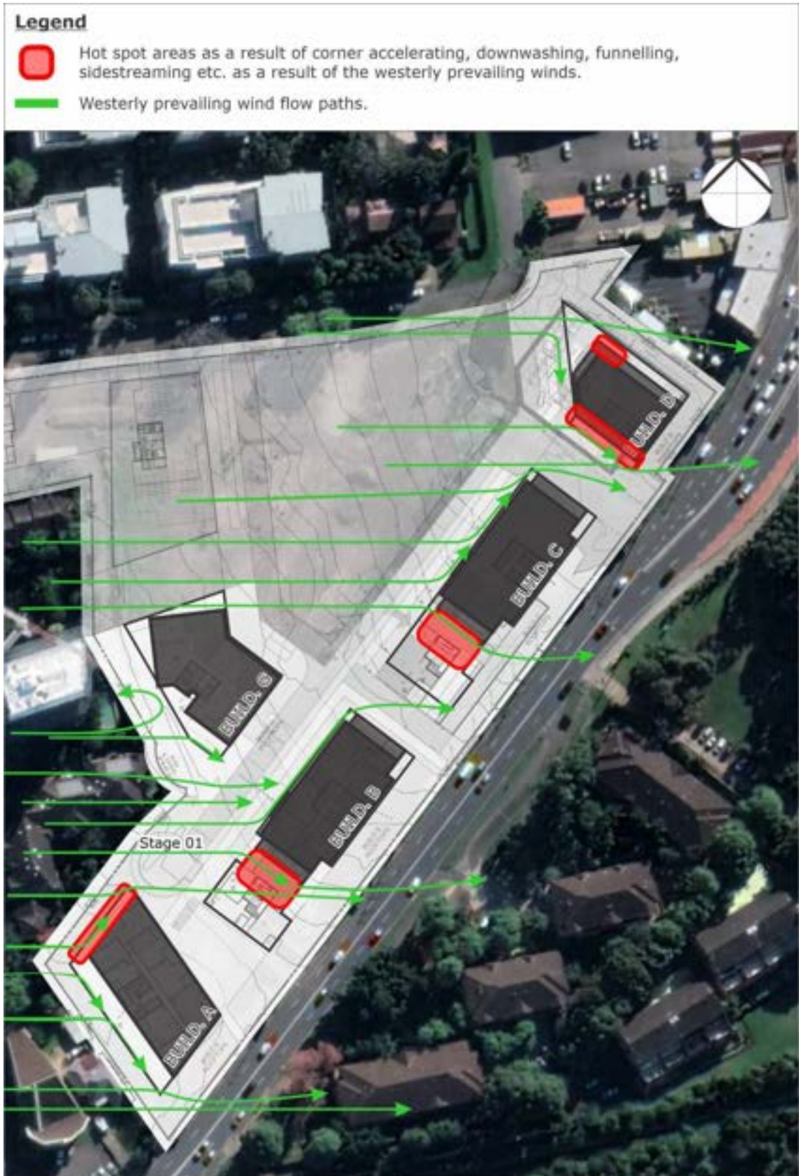
Figure 13: Westerly Wind Flow Hotspots Future Built Form in Stage 01 - Podium Level Plan
