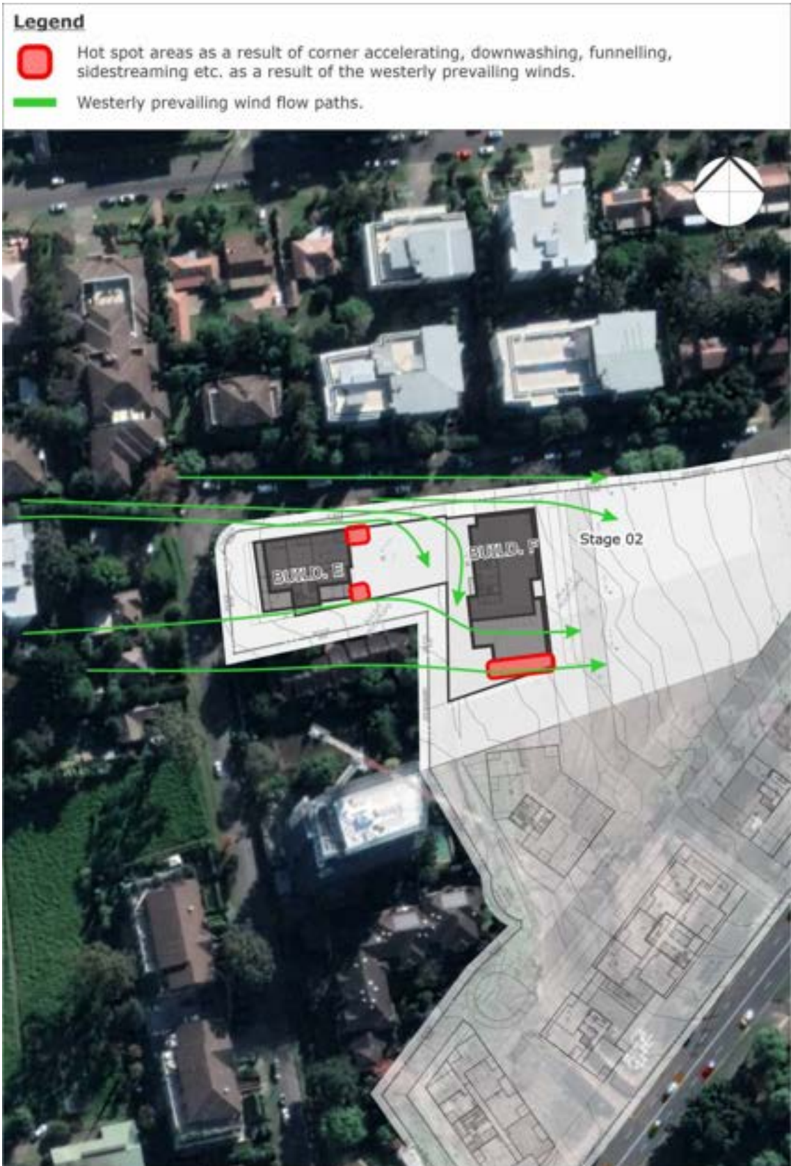
Figure 15: Westerly Wind Flow Hotspots Future Built Form in Stage 02 - Podium Level Plan
