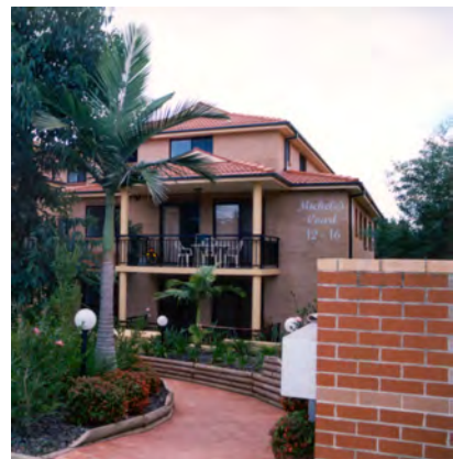
Ensure that balconies have enough depth to accommodate a table and chairs.
