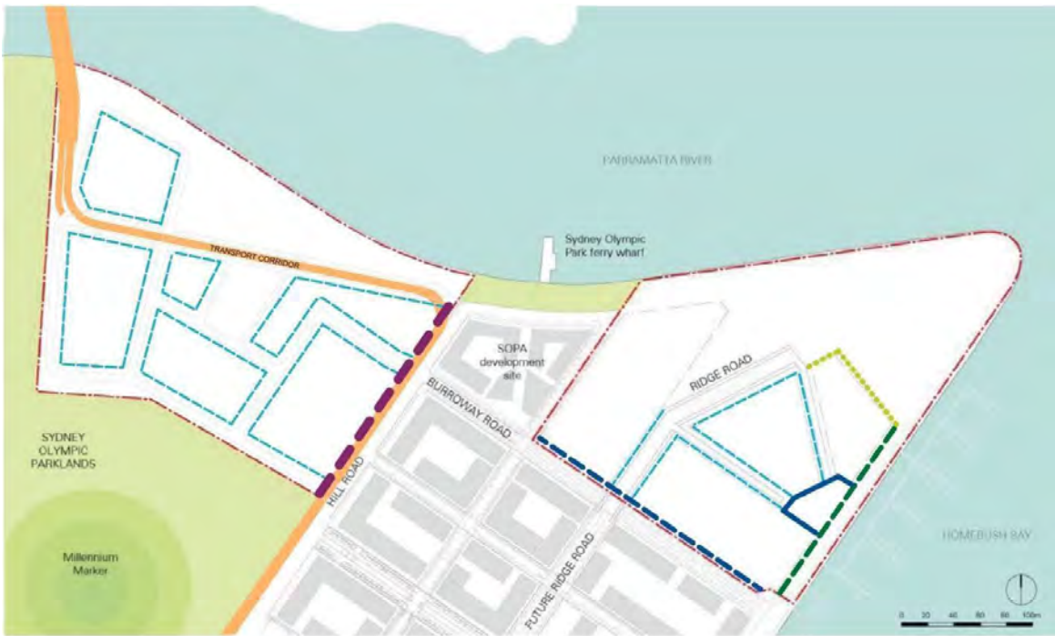
Legend Site boundary (red dashed line) 5m (blue dashed line) 5m to park edge (yellow dashed line) 25m (green dashed line) 3-5m to road (cyan dashed line) 0m (solid blue line) Indicative Transport Corridor (orange solid line)
