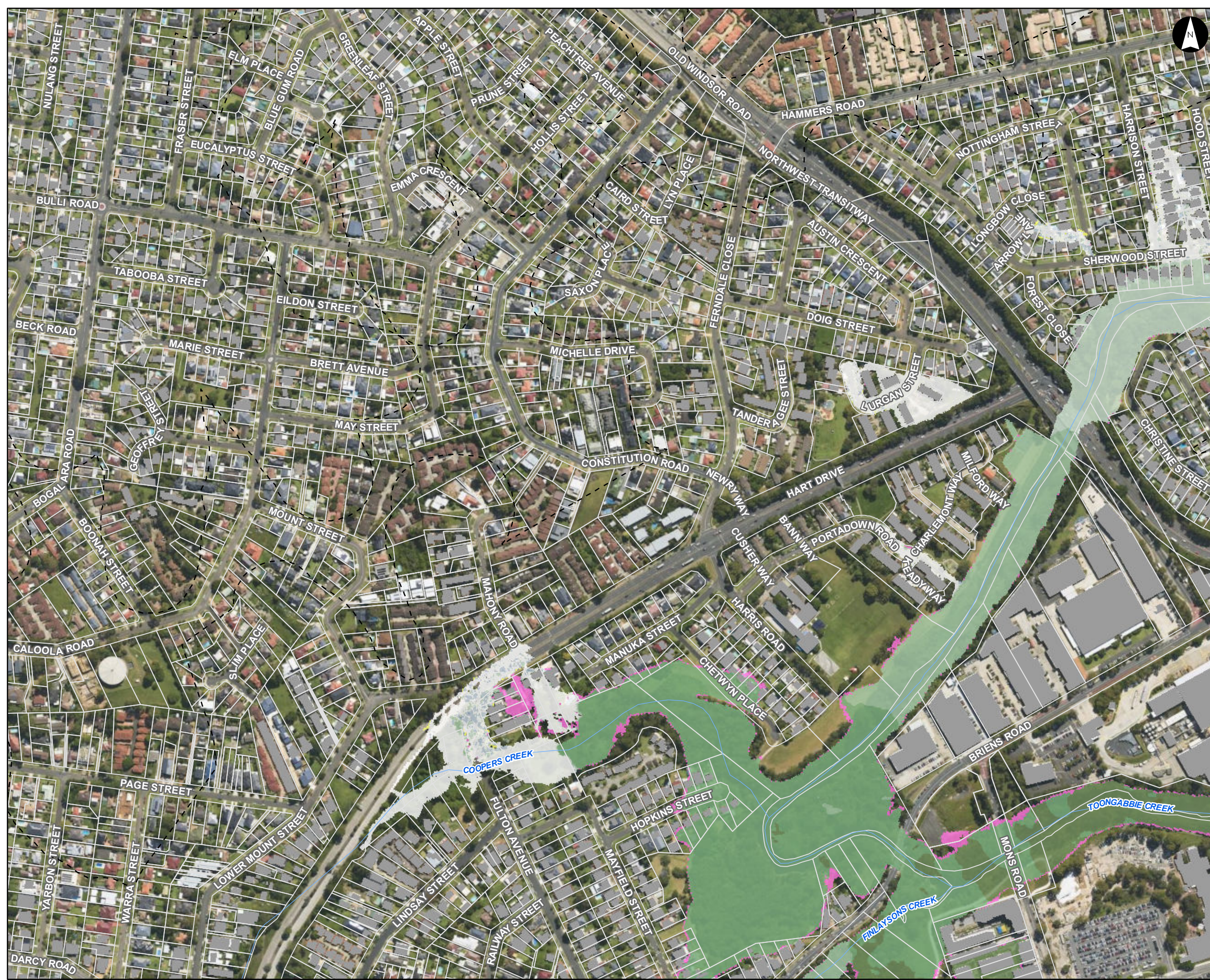
Sensitivity Analysis SS7 Basin Removal FFA 1% AEP Peak Flood Level Difference Plot
