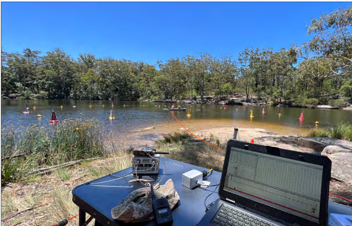
Figure 2. MSR setup for Line 2. Picture taken from seismograph operator looking out towards air gun operators. Note the orange polyline representing the seismic array.
