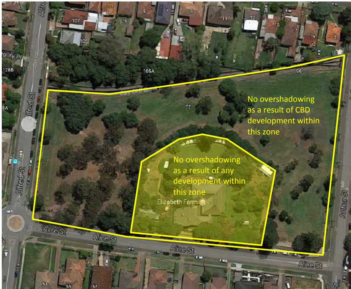
Figure 40: Elizabeth Farm Cottage solar access curtilage. The core of the site including the cottage and garden must not be subjected to any additional overshadowing.
