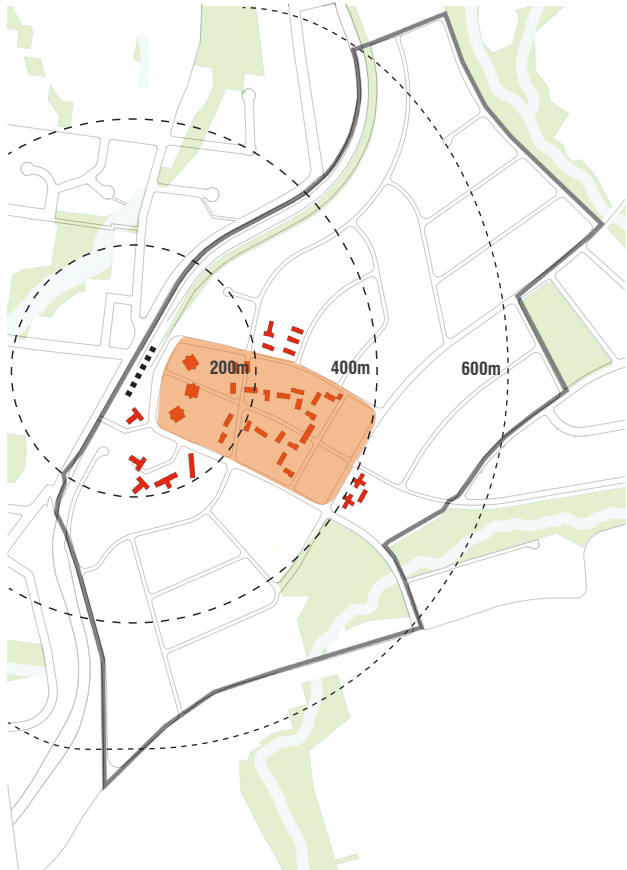
Higher densities located in the core to facilitate renewal of ageing social housing and shops.
