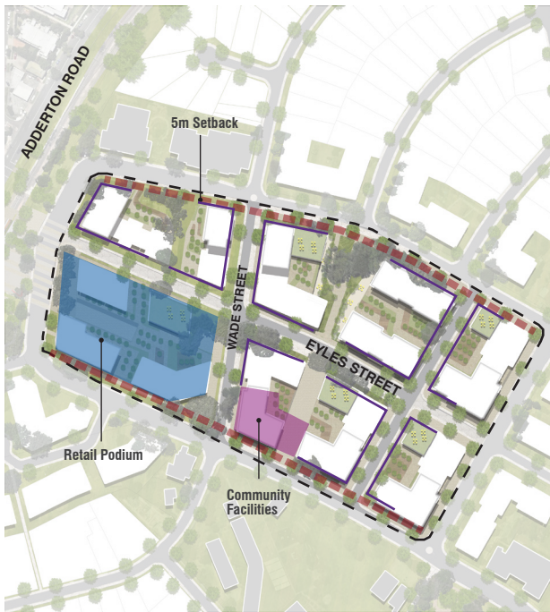
Key Plan shows indicative built form within part of the Mixed Use Core and High Density Housing
