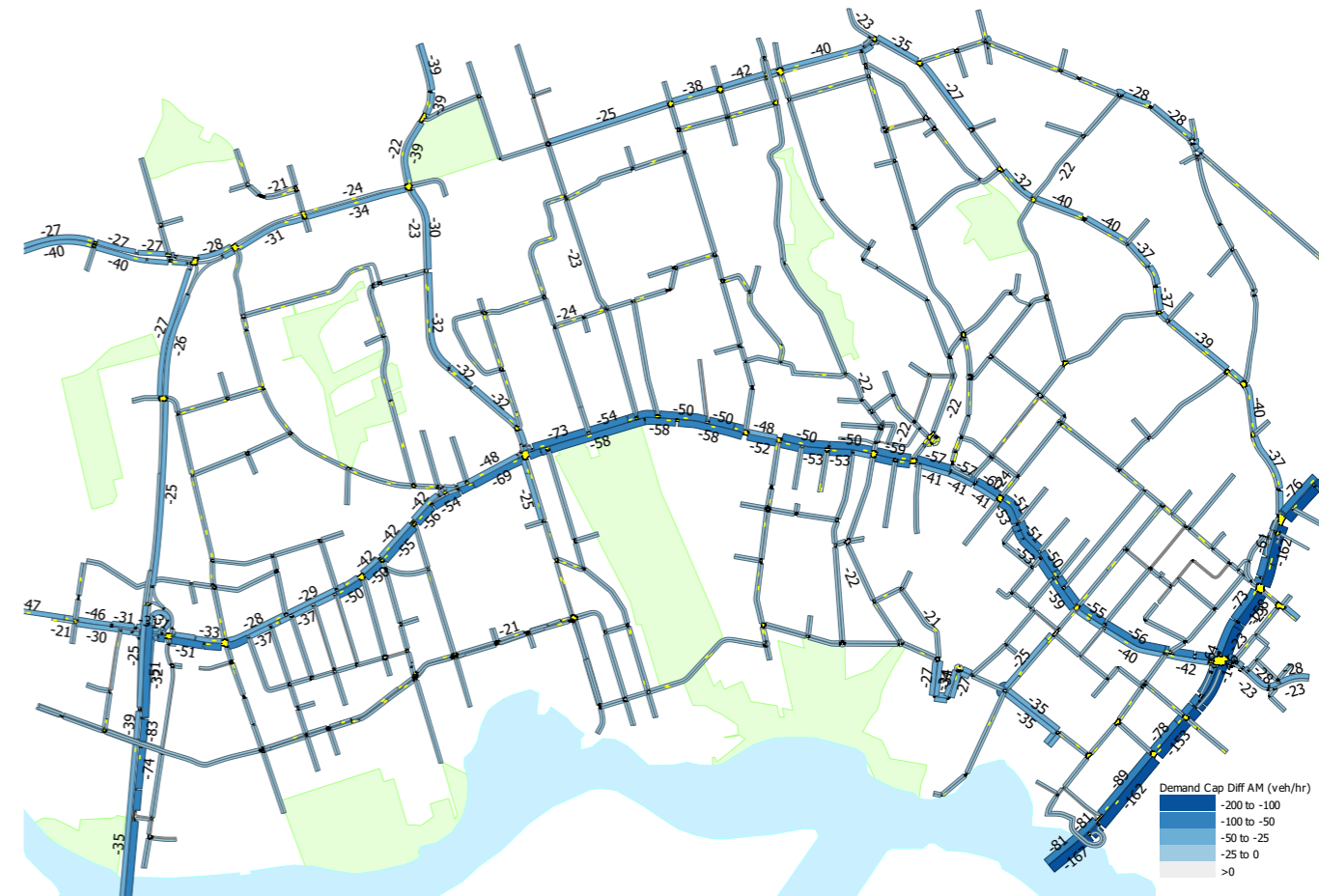
Figure 5.12 Difference plot comparing capped and uncapped 2036 AM demand (average hourly flows over 4-hour modelled period)
