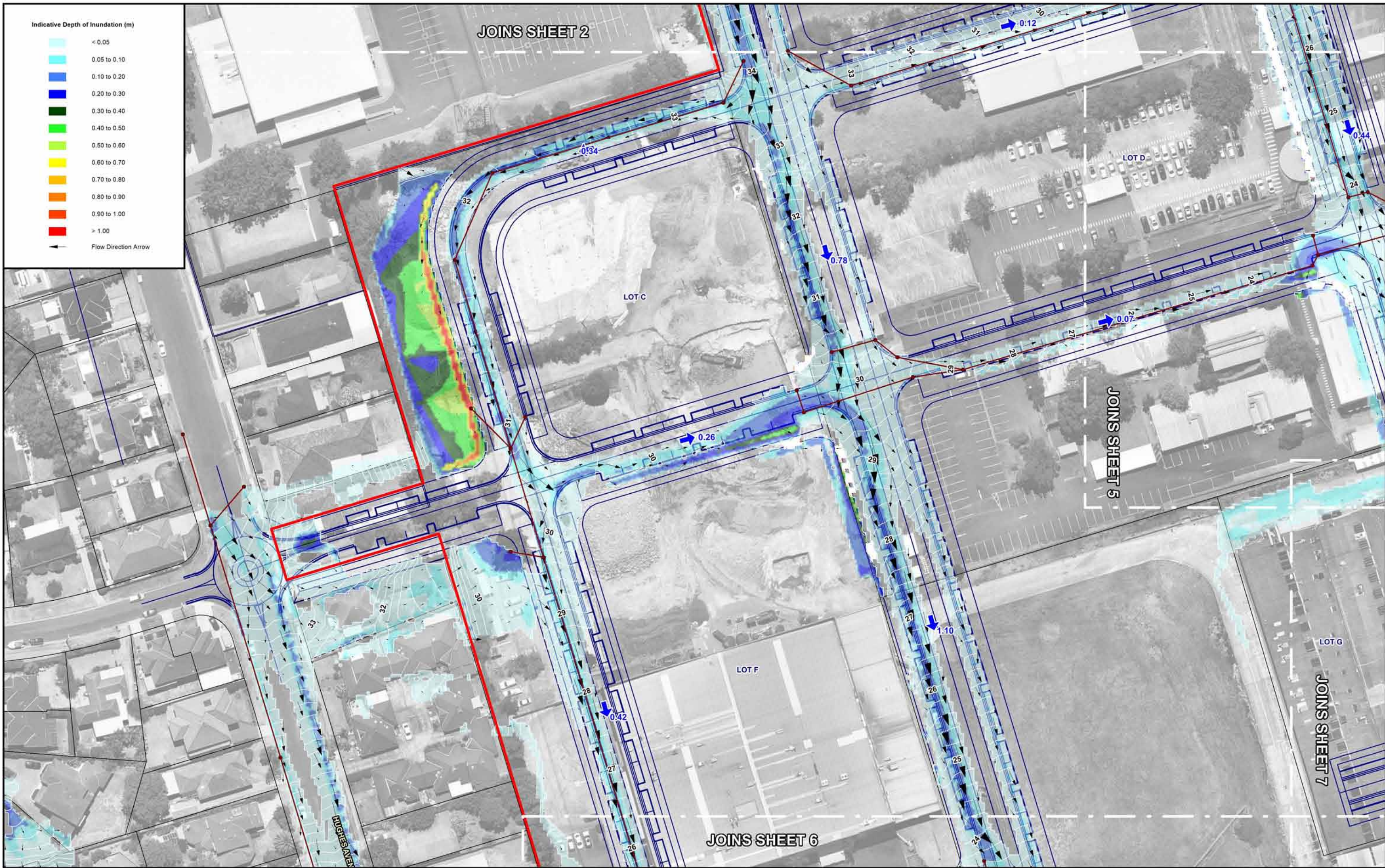
Figure 6 (Sheet 4 of 7) INDICATIVE EXTENT AND DEPTH OF INUNDATION POST-VRS AND PP DEVELOPMENT AND COMPLETE BLOCKAGE CONDITIONS - 1% AEP
