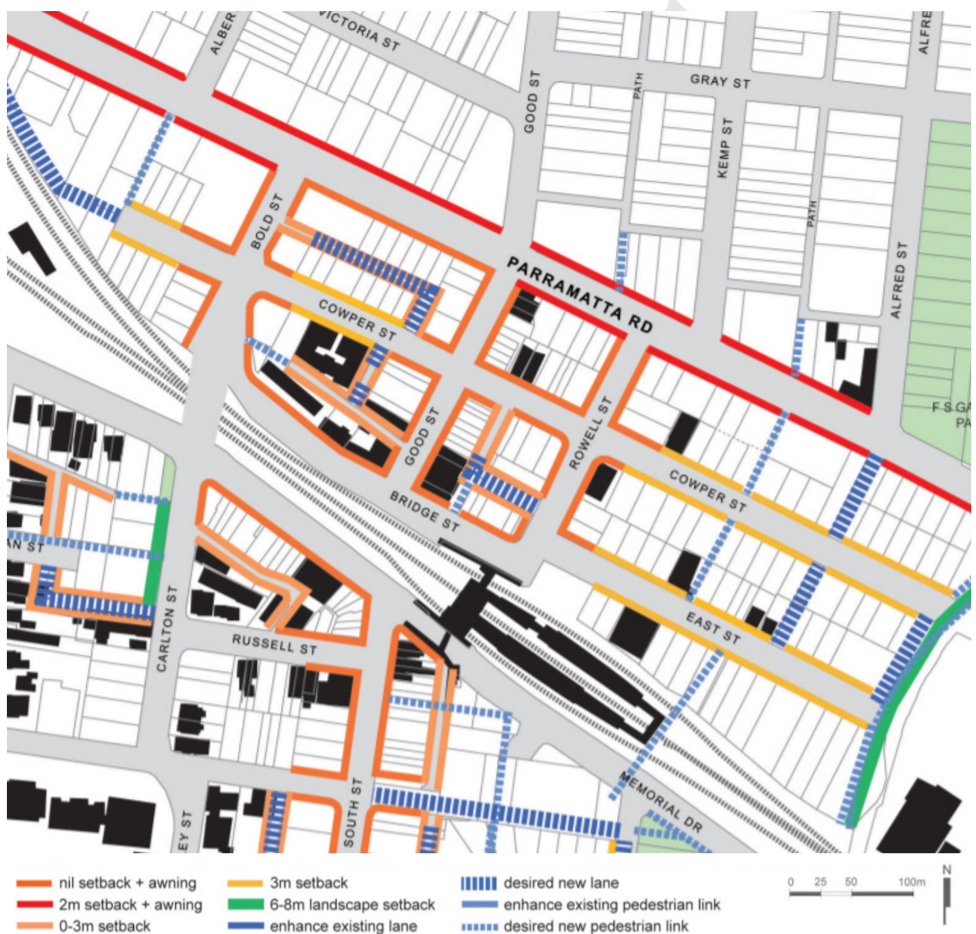
Above: Building Setbacks, Pedestrian Links and Laneways for Granville Town Centre as identified in the DCP 2011
