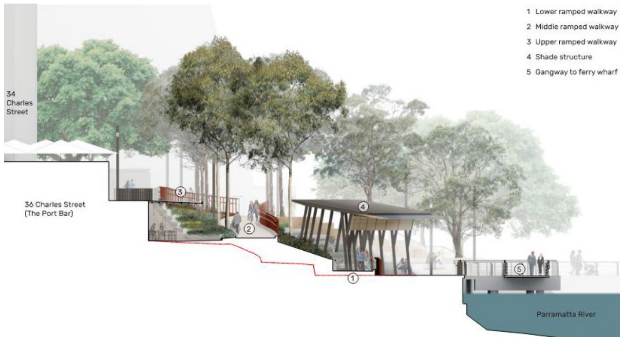
Figure 6 Three ramped walkways traverse the height change between the city and the riverfront.
