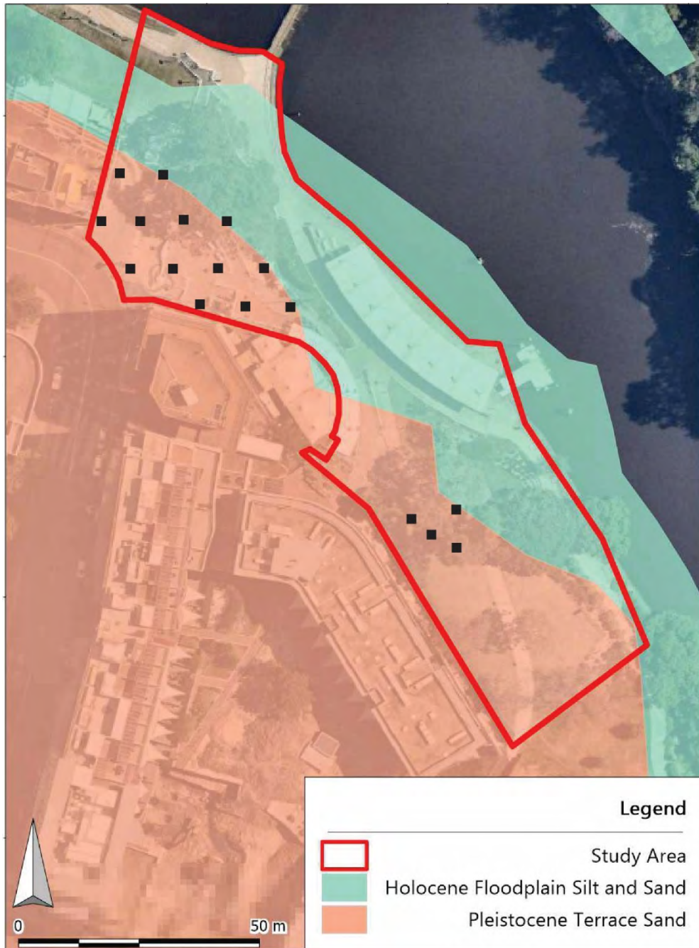
Figure 8.3: Indicative layout of maximum number of Phase 1 test trenches at 10m spacing.
