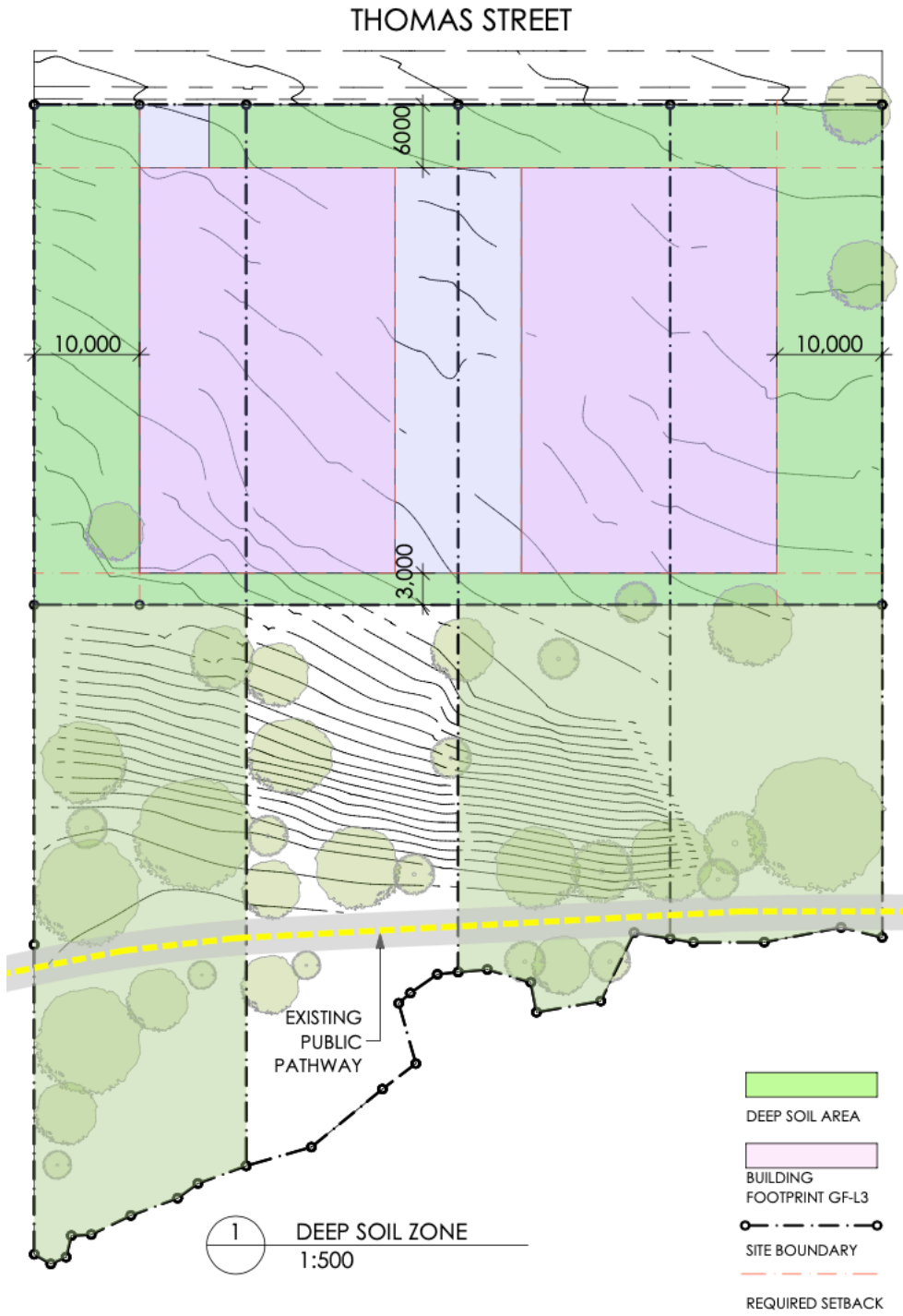
Figure 4.1.9.16 Area 5 Deep Soil Zone
