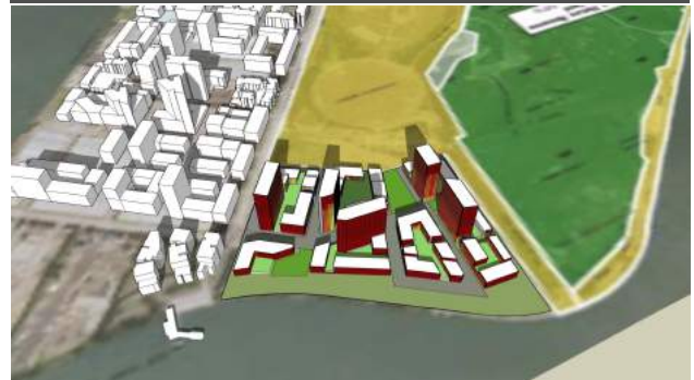
URBAN GROWTH SCHEME – SOLAR GAIN AT 11 AM
