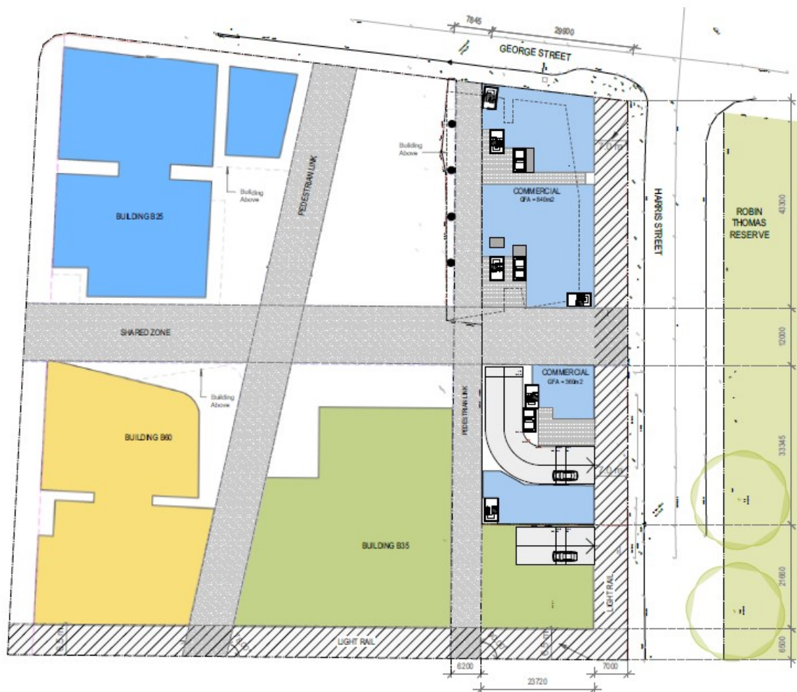
Figure 5: Ground floor plan indicating relationship with Cumberland Industries site. (Source: Applicant's Urban Design Report)
