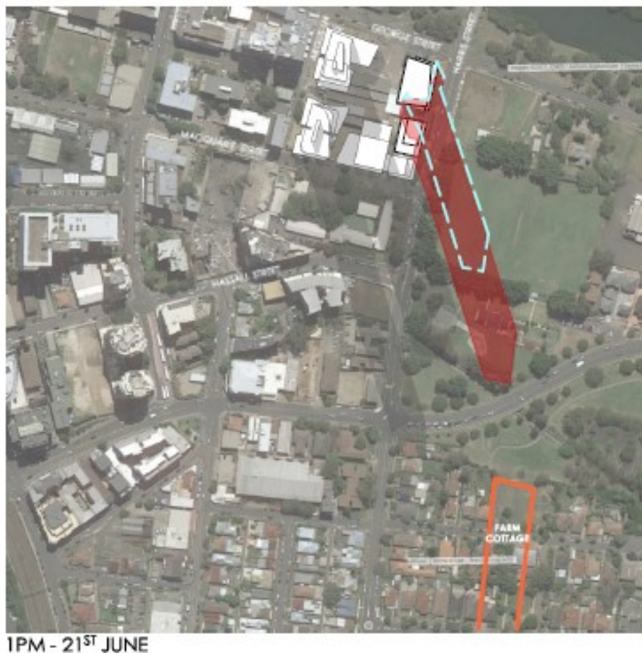
Figure 8: Shadows cast by the development at 1pm on 21 June based on FSR of 13.5:1 and Height of 166 metres (Source: Applicant's Urban Design Report)
