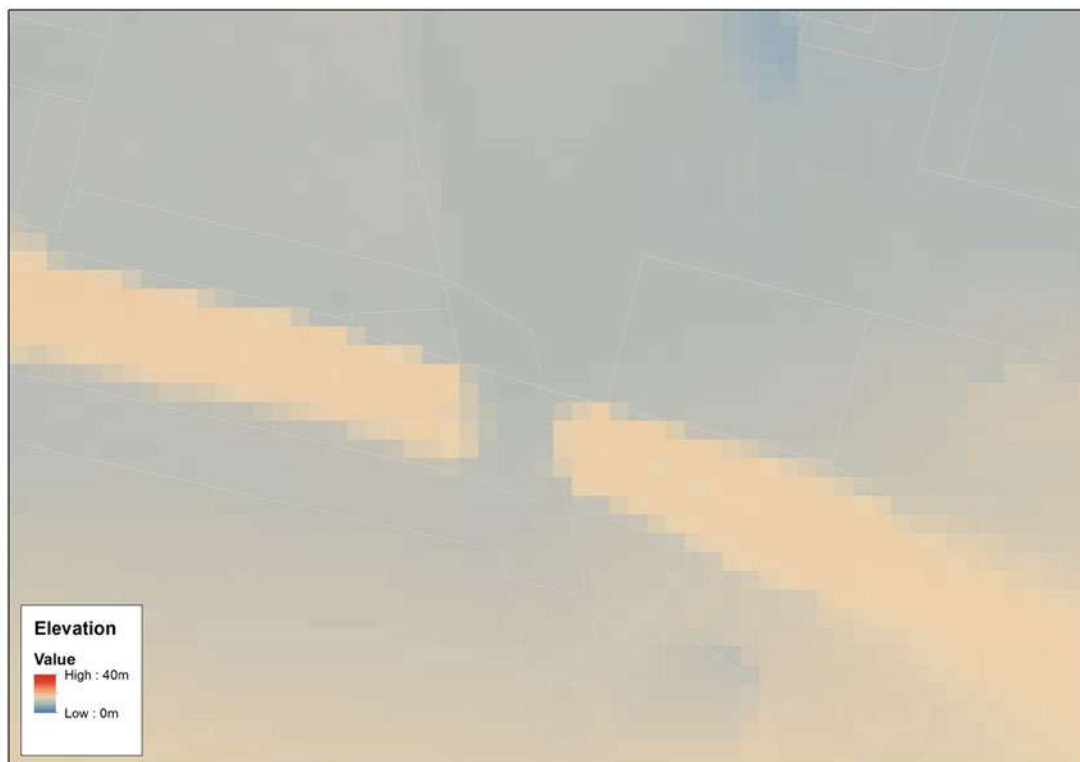
Figure 4 - Digital Elevation Model at the Church Street railway overbridge abutment. Note the clear definition of individual 5x5m "pixels". Map Scale 1:1,000 @ A4 (scaled to 50% in this document)
