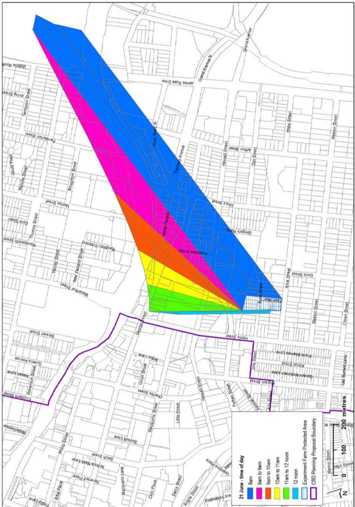
Figure 20 - Revised Sun Access Protection Surface for the period 8am to 12-midday on 21 June
