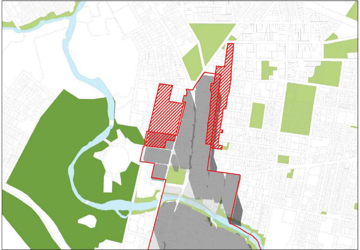
Figure 64 - Current and Proposed Controls overshadowing - 21 June - 1pm
