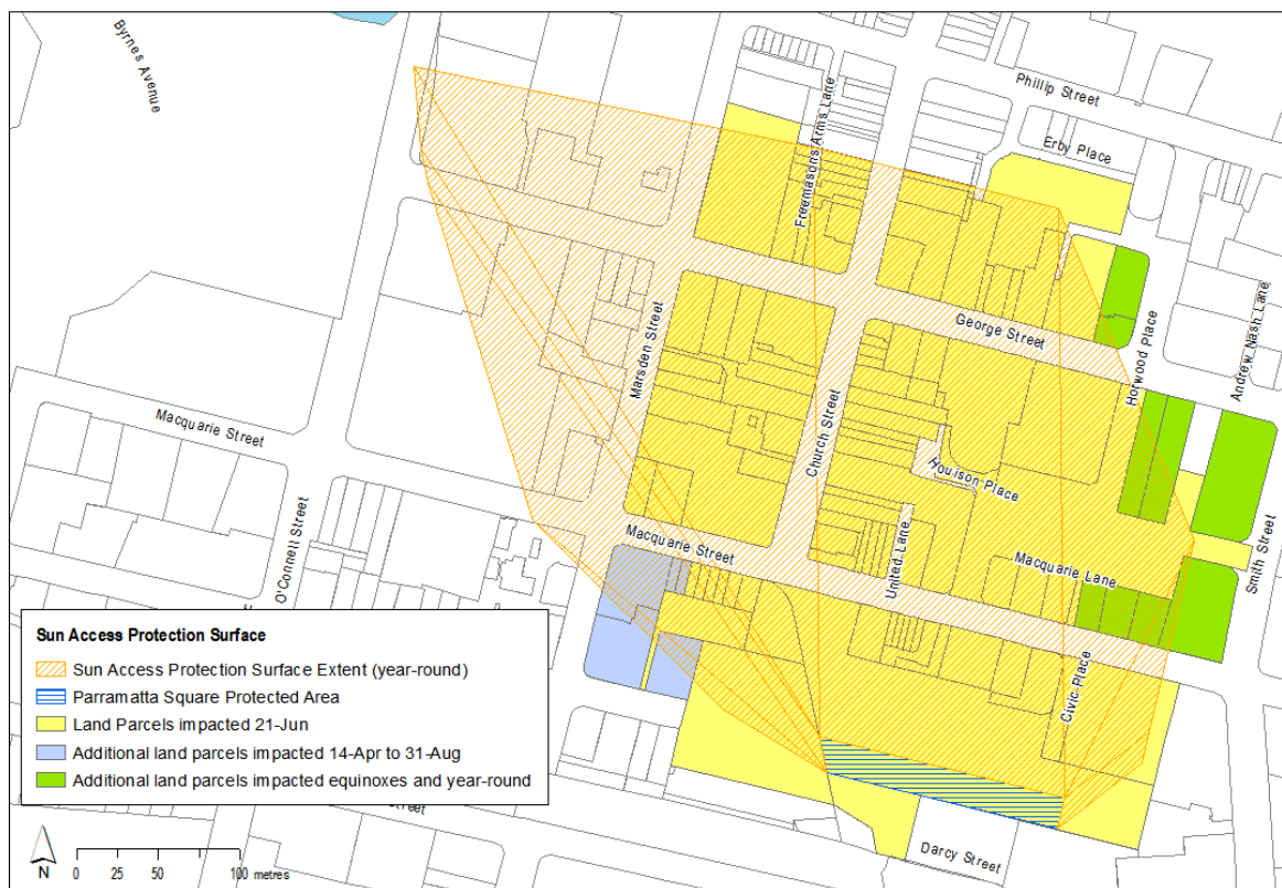
Figure 31 - Land parcels potentially impacted by scenarios for Parramatta Square Sun Access Protection surface
