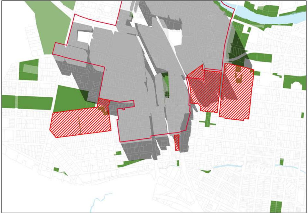
Figure 52 - Current and Proposed Controls overshadowing - 21 June - 1:30pm
