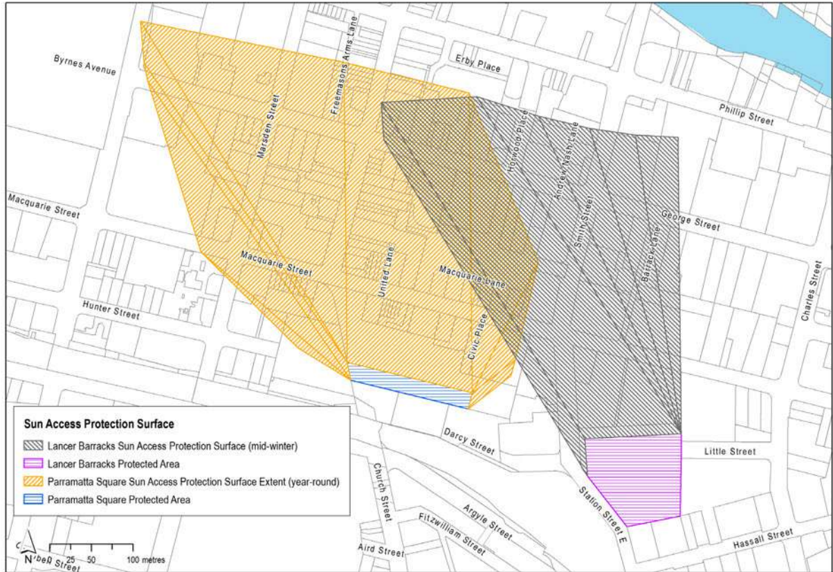
Figure 32 - Overlapping Sun Access Protection Surfaces for Parramatta Square and Lancer Barracks
