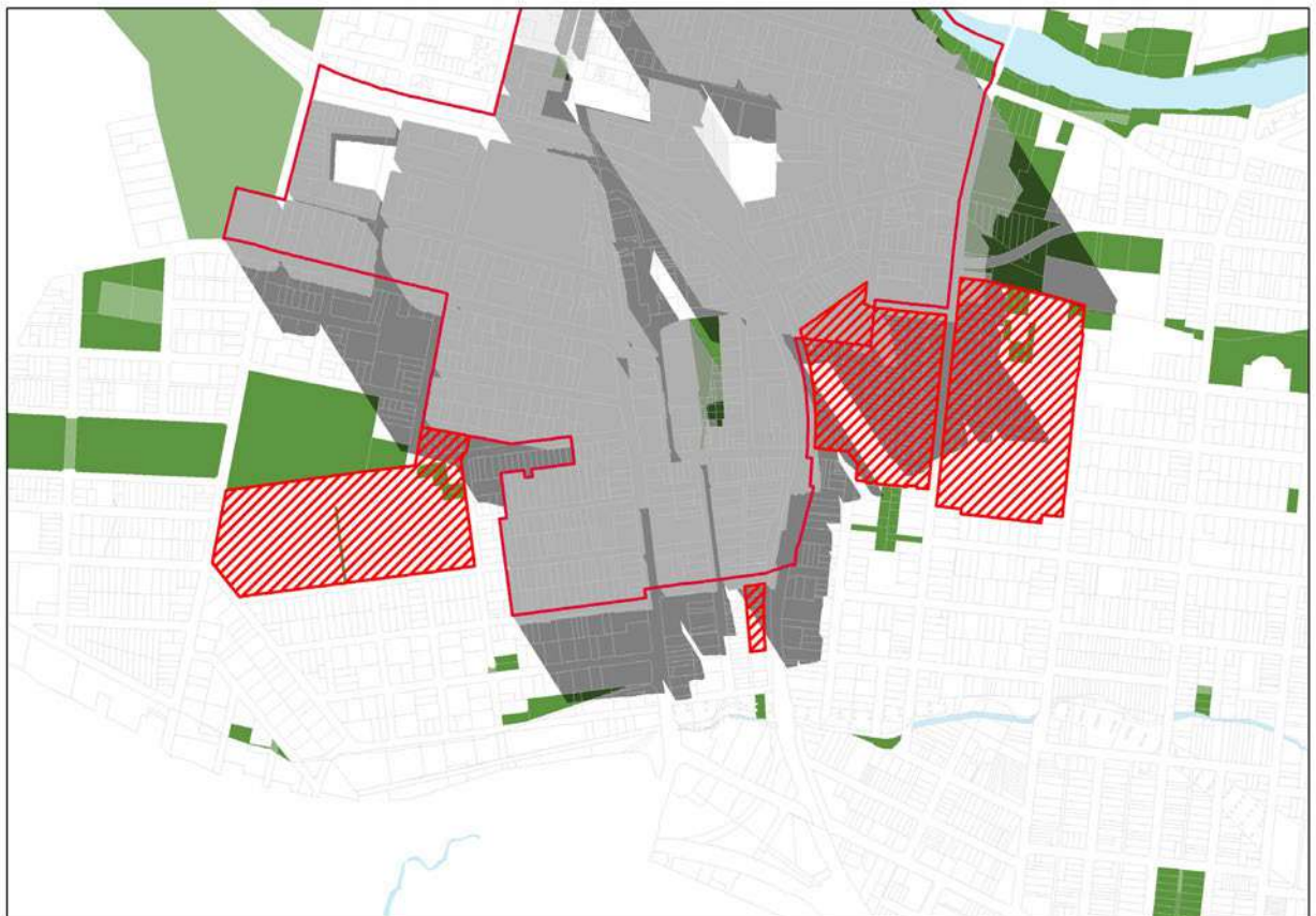
Figure 53 - Current and Proposed Controls overshadowing - 21 June - 2pm
