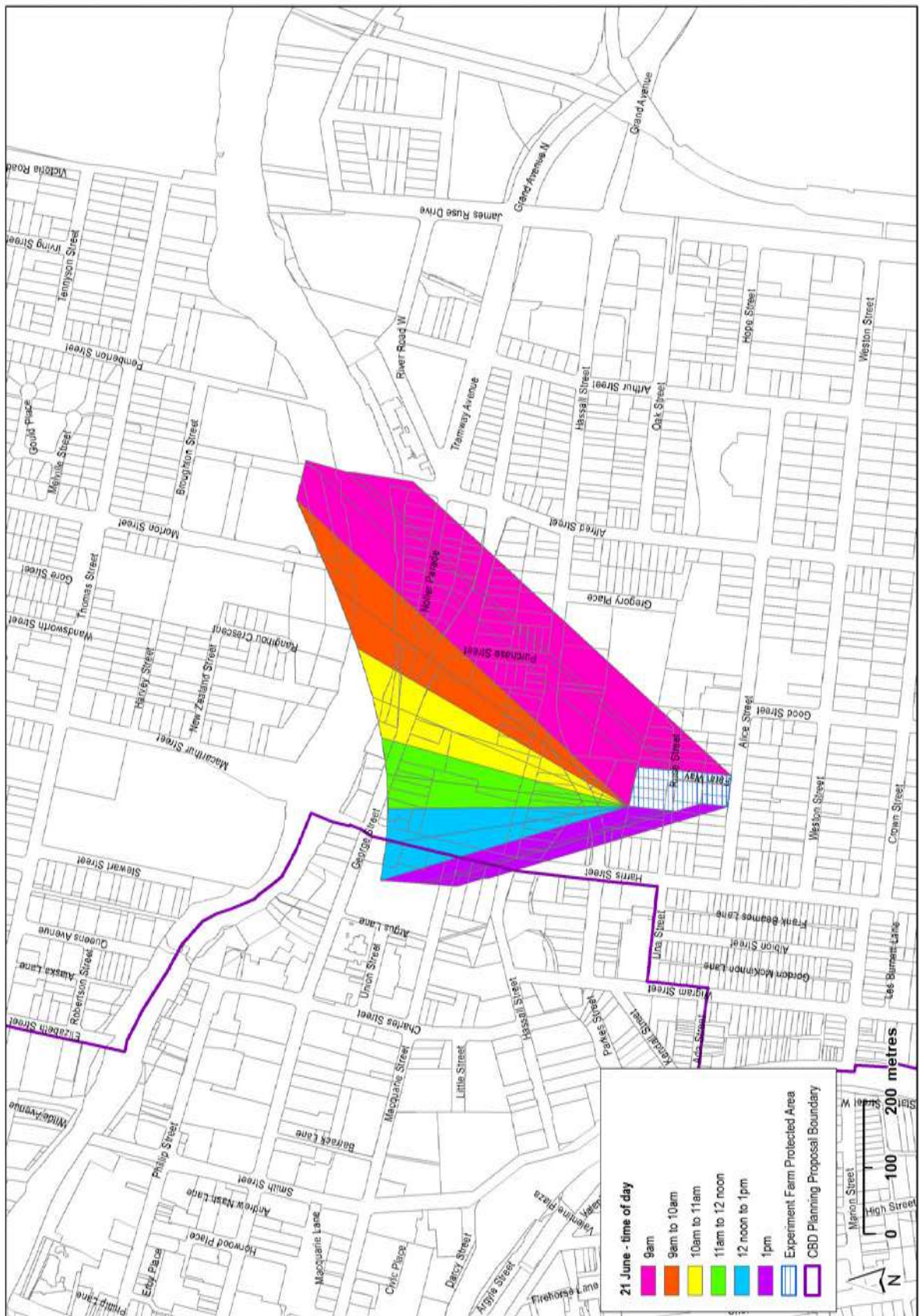
Figure 21 - Revised Sun Access Protection Surface for the period 9am to 1pm on 21 June
