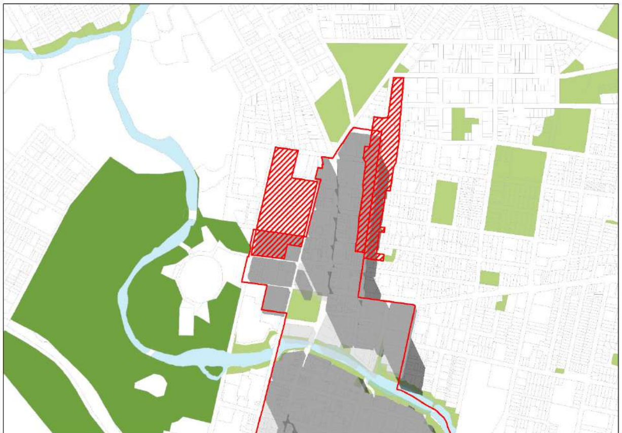
Figure 65 - Current and Proposed Controls overshadowing - 21 June - 1:30pm
