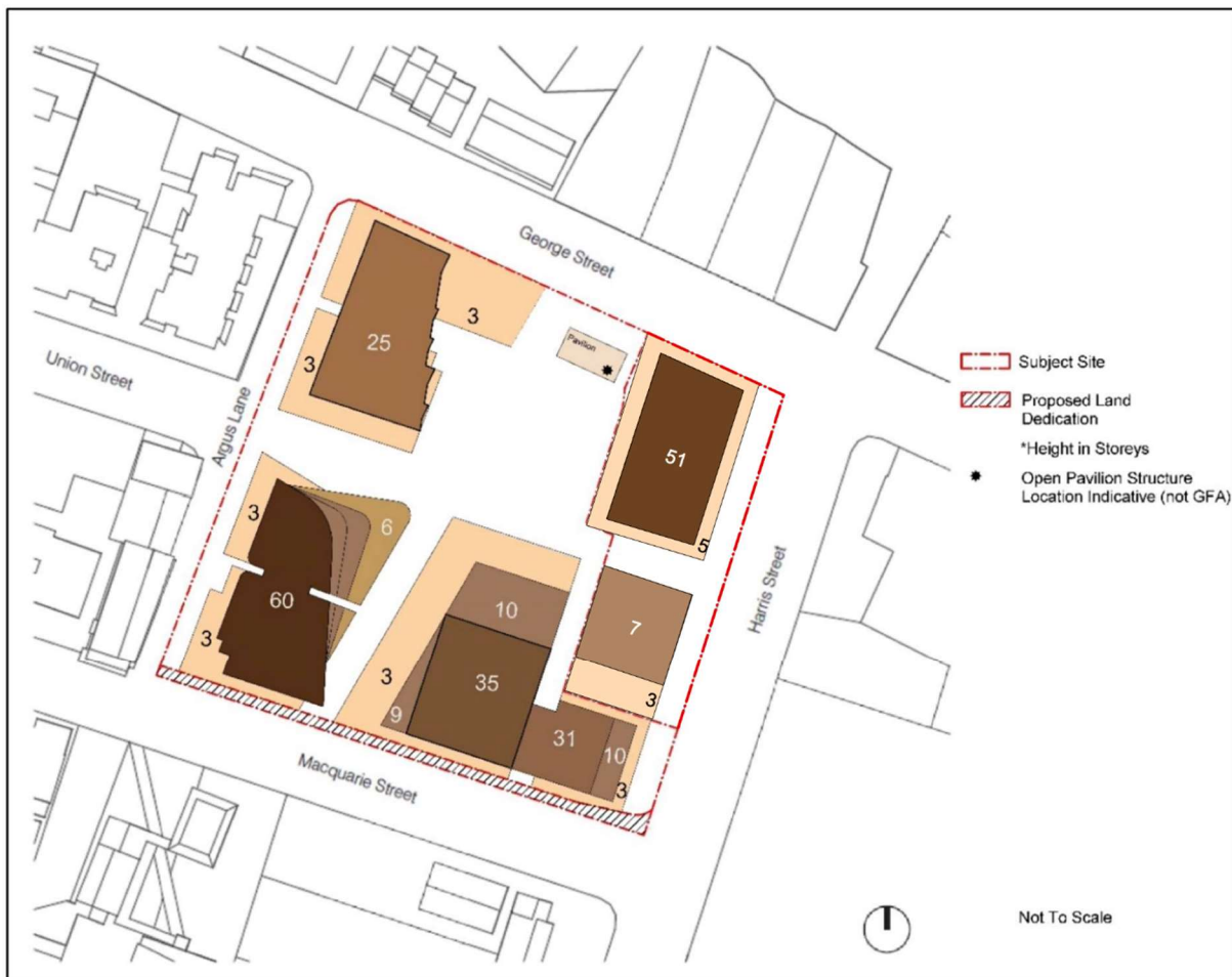
Figure 4.3.3.7.26 – Control diagram: Height of buildings in storeys on former Cumberland Media Site
