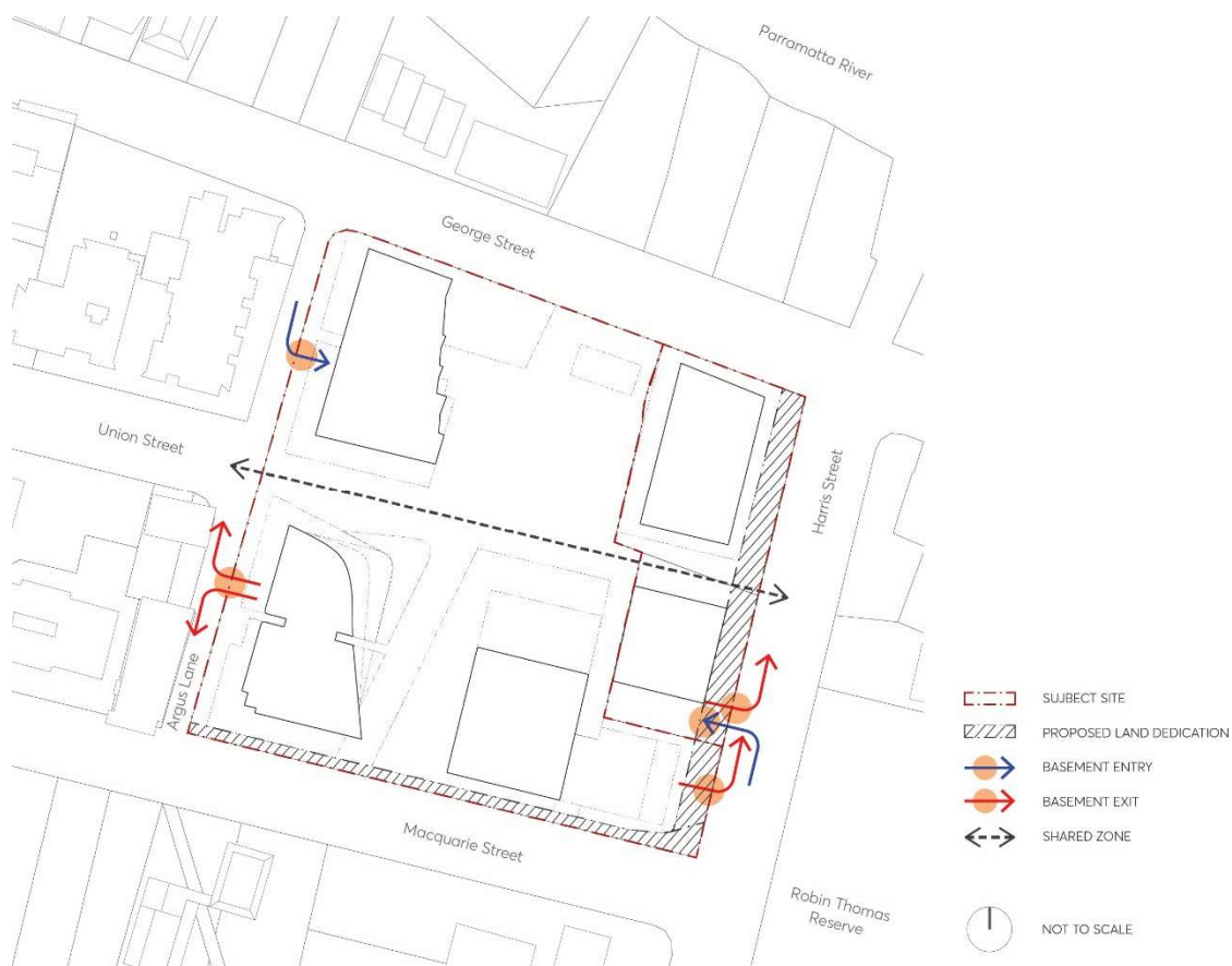
Figure 4.3.3.7.30 – Control diagram: Vehicular Access and Servicing
