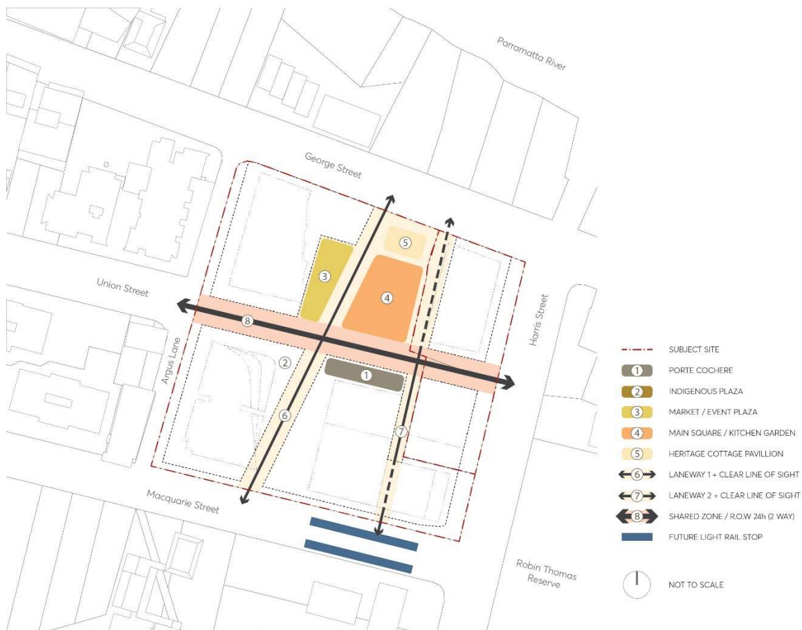
Figure 4.3.3.7.31 – Control diagram: Pedestrian links and shared zones
