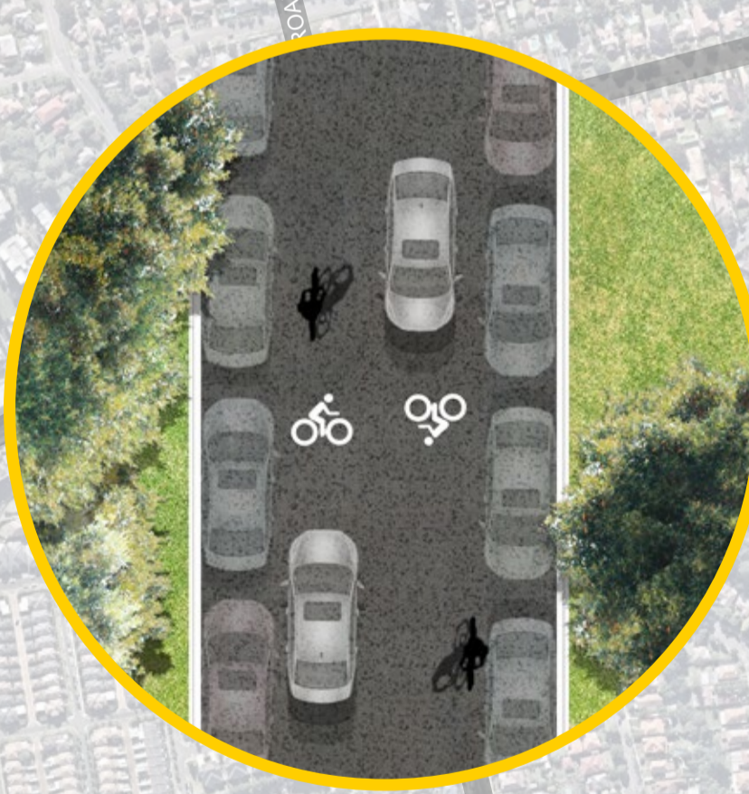
PROPOSED MIXED TRAFFIC Proposed mixed traffic: bike logos painted on road and no change to current conditions.
