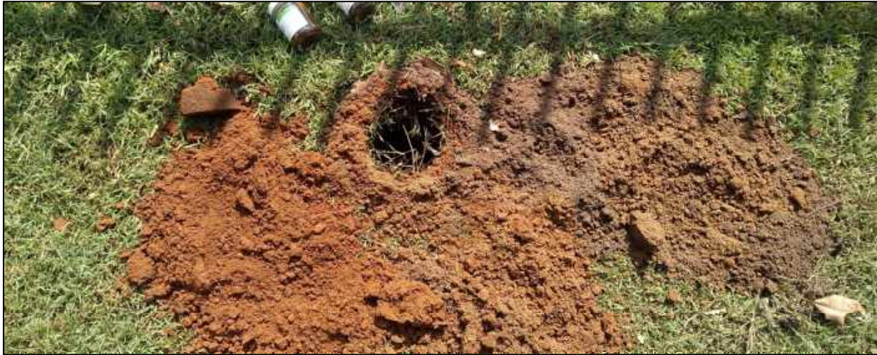
Photograph 1. Sandy CLAY - in situ soil materials located at HA03.
