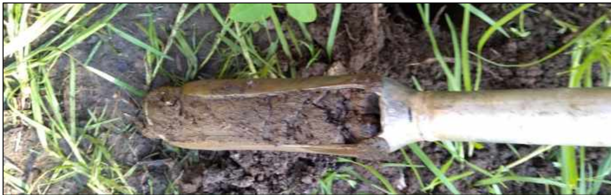
Photograph 3. Silty CLAY - in situ soil materials located at HA01.
