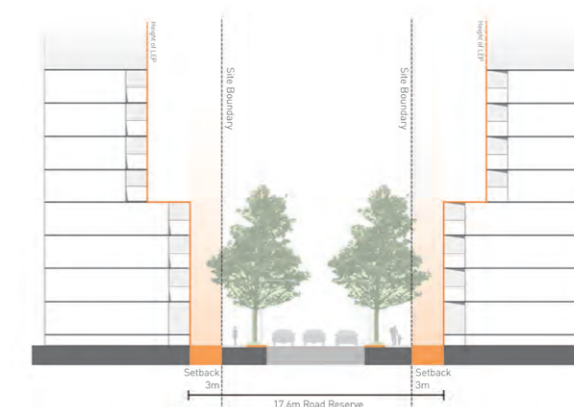
Figure 4.8 : Internal road sections - southern precinct
