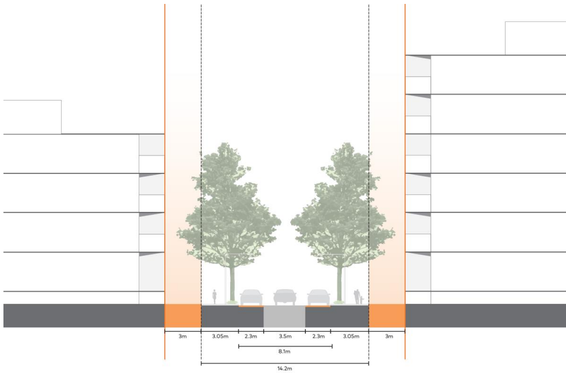
Figure 70: Setbacks from 14.2m road reserve within the proposed local roads. (Source: COX)
