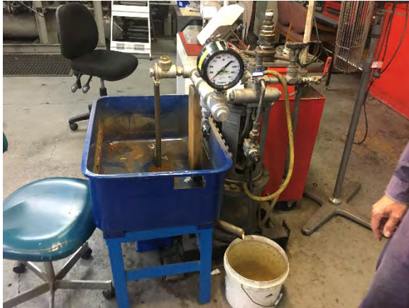
Photo 7. Pressure testing valves with water.
