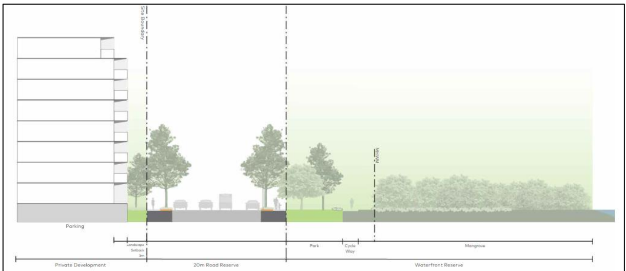
Figure 30: Foreshore Road and Open Space Interface
