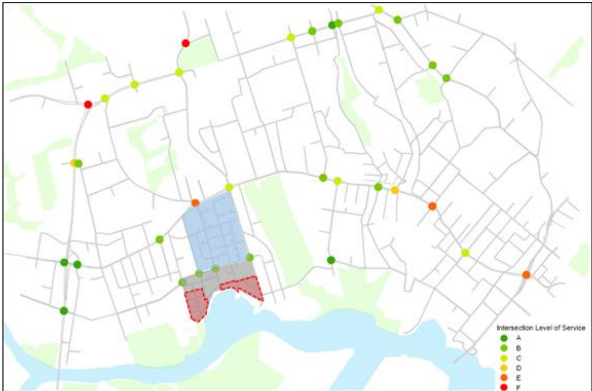
Figure 20: Future PM Peak Hour Intersection Operations
