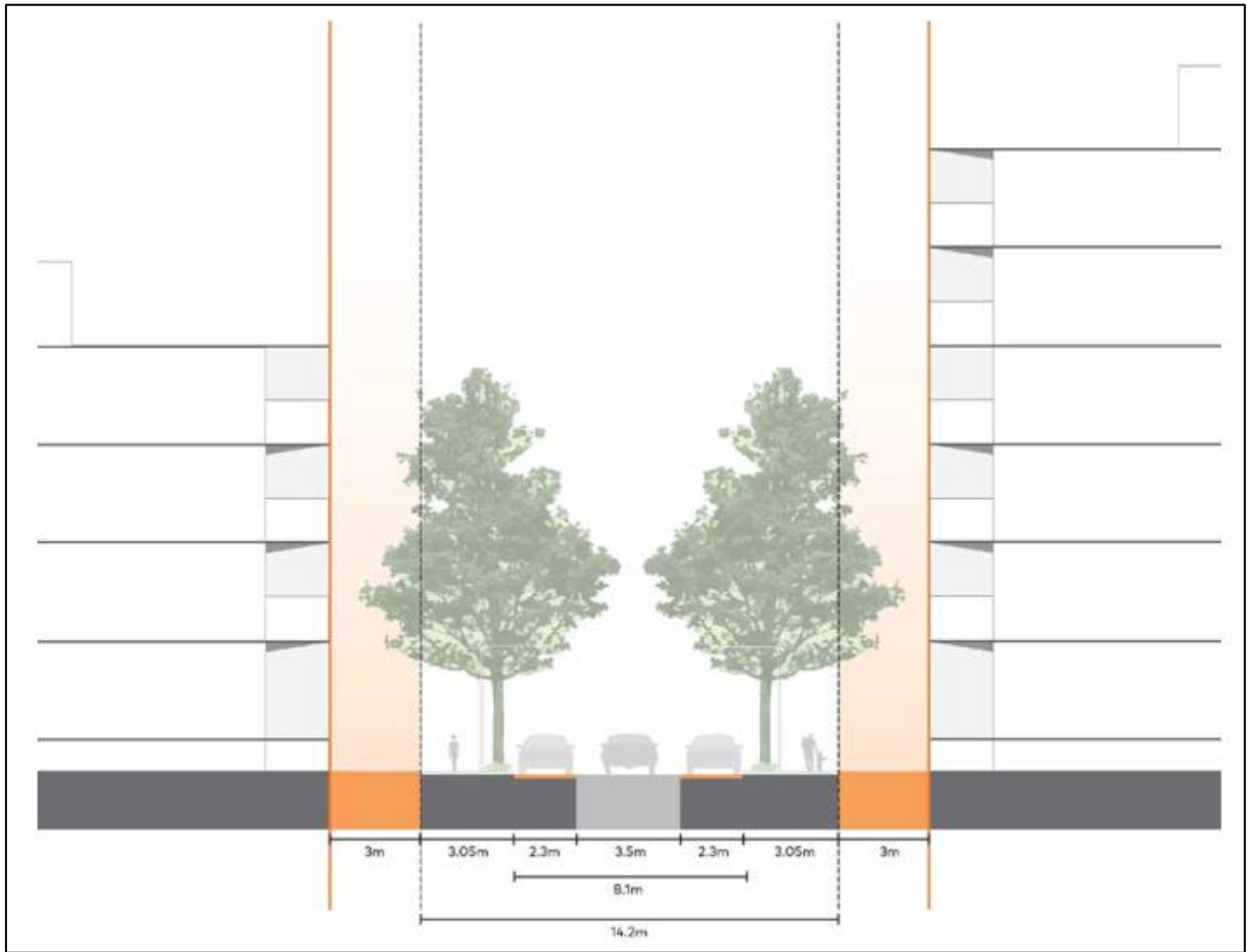
Figure 28: Local Road Design Profile – 14.2m Road
