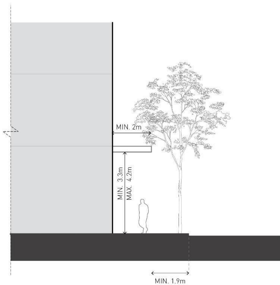
Figure 18 - Typical Awning Condition with Street Trees
