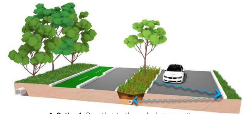
1. **Option A:** Directly into the kerb drainage pits.
