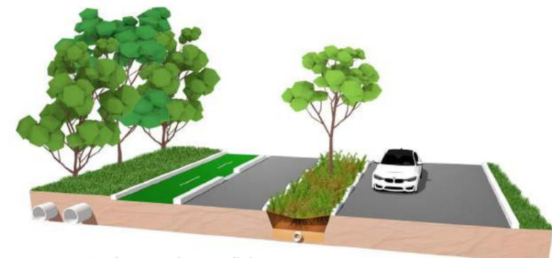
4: Duplicating the parallel stormwater pipe.
